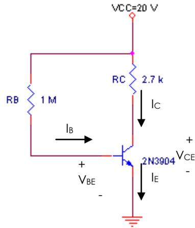
2. Using  $\beta = 100$ , calculate the theoretical values of  $I_E$ ,  $I_C$ ,  $I_B$  and  $V_{CE}$ . From the values of the currents, calculate the values of  $V_B$ ,  $V_E$  and  $V_C$ .
