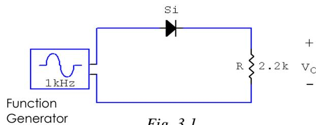
3. Reverse the diode of circuit of *Fig. 3.1*. Sketch the output waveform across the resistor. Measure and record the DC level of the output voltage.
